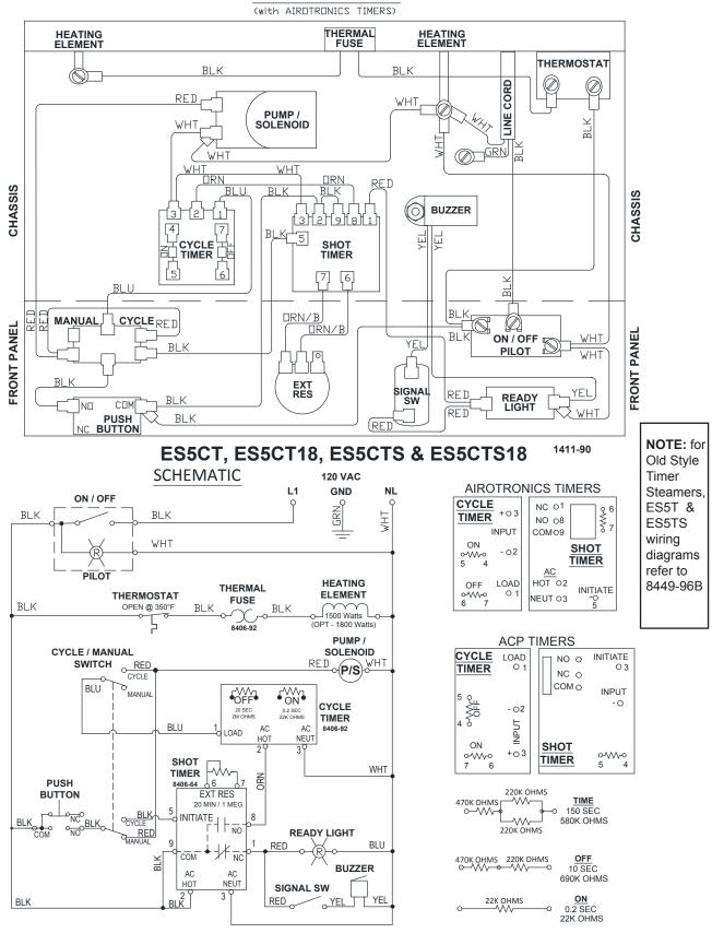
Figure 2B Wiring Diagrams for ES5 Series Steamers - ES5CT, ES5CT18, ES5CTS & ES5CTS18 with Mechanical Timer Note: ES5 1800 Series Steamers have an 1800 watt heating element
