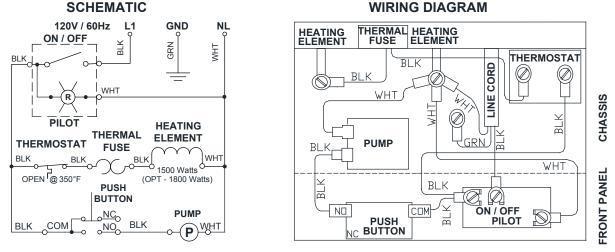
Figure 2A Wiring Diagrams for ES5 Series Steamers - ES5M, ES5M18, ES5MT, ES5PB, ES5PB18, ES5PBS & ES5PBS18 Note: ES5 1800 Series Steamers have an 1800 watt heating element
